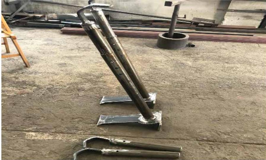
**Figure 1.** Adjustable eccentric hook device
